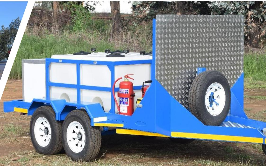
The versatile service trailer is equipped with a diesel compressor delivering 6.5 bar of pressure to drive the reliable double diaphragm type fluid pumps.
