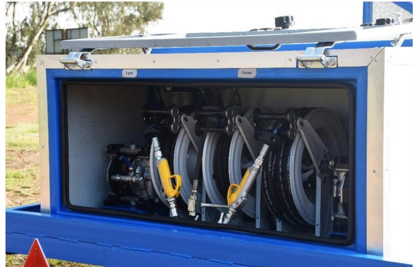
Spring return hose reels ensure safe and easy retractable 15m hoses while keeping things nice and tidy while travelling.
